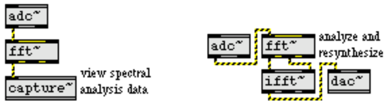
Fast Fourier transform of an audio signal
